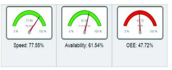
Real-Time feedback is provided to the users through a range of auto-generated reports and displays. This information can also be displayed via big screens within the plant to provide visual feedback to staff. It also has an ANDON capability where abnormalities can be made visible.
